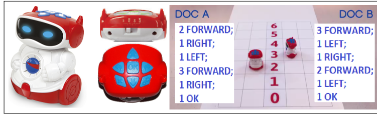
Fig. 2: Left : Robot Doc with its keyboard and modes selector. Right : Educational activity: commutative properties of the sum on the line of numbers.
