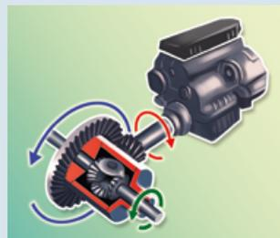
The pinion gear transfers the engine's power to the differential and, as a result, to the axle shafts, turning the wheels.
