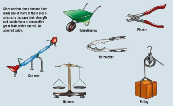
A simple machine is an instrument that allows for balancing and overcoming **RESISTANCE** (weight, resistance force = **R**) with **EFFORT** (manpower = **E**).
