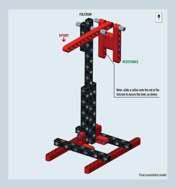
Find the equilibrium of this type of mechanical device: position the weight (RESISTANCE) on one side of the lever and gently press down with your hand (EFFORT) on the other side.
